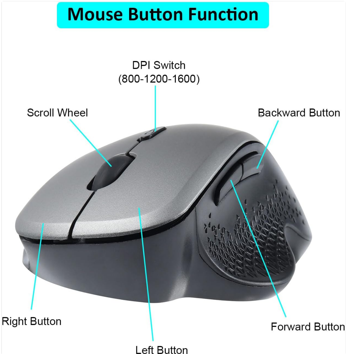
Image 2: An illustration detailing the location and function of each button on the vertical mouse.
