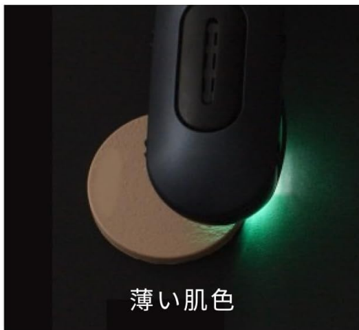
Figure 2.3: Illustration of the focus sensor detecting skin tone and adjusting power.
