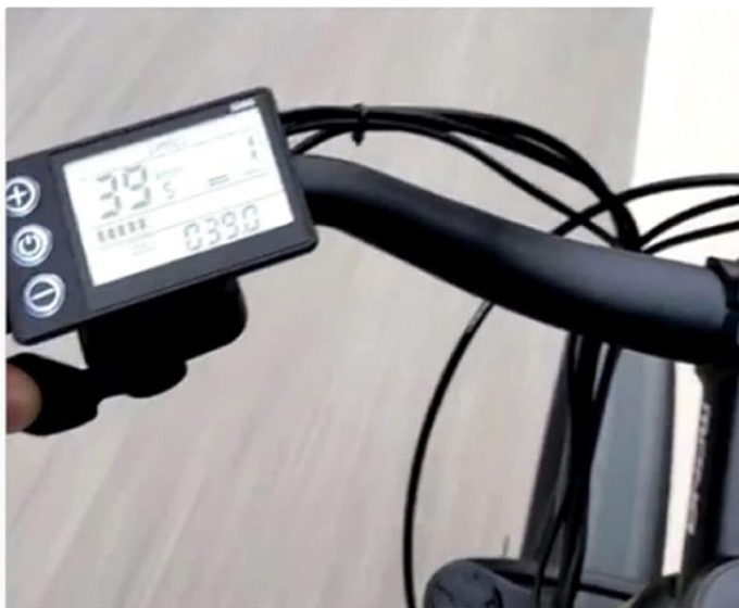
Figure 4: Front view of the display, showing speed, assist level, battery indicator, and trip distance.
