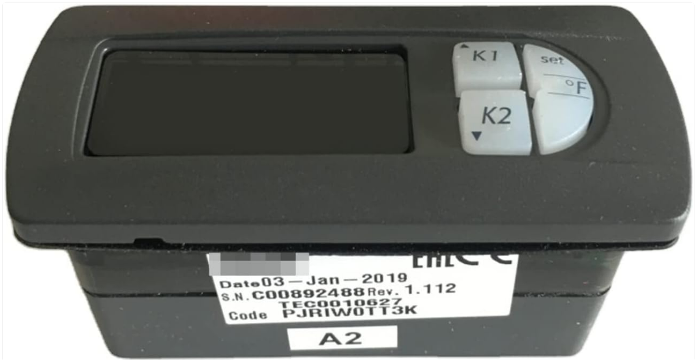
Figure 1: Front view of the PJRIW0TT3K Temperature Controller, showing the digital display on the left and control buttons (K1, K2, set, °F) on the right. The model code "PJRIW0TT3K" is visible on a label at the bottom.
