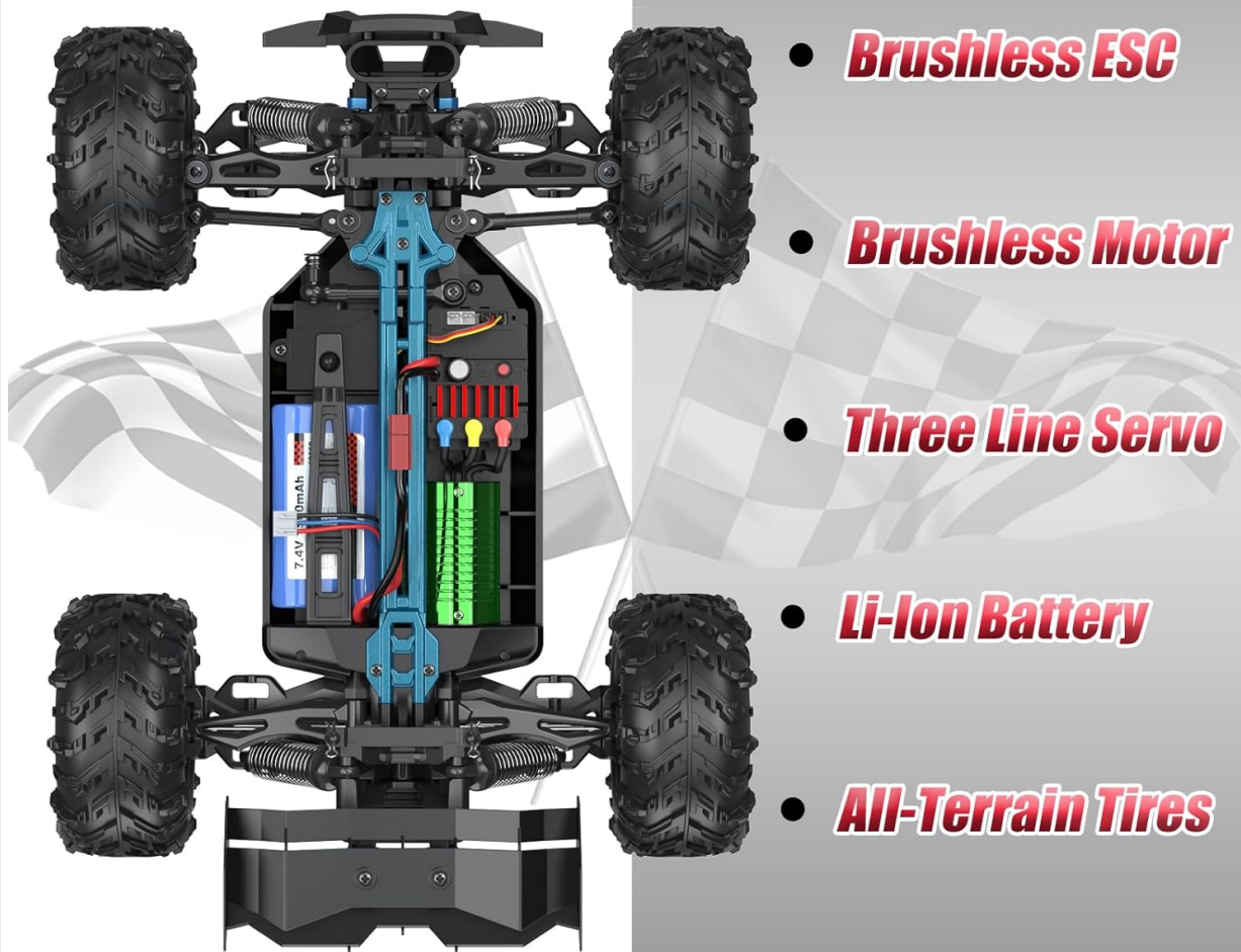
Image 3.1: Overview of the RC truck's internal components, including the brushless ESC, brushless motor, three-line servo, Li-ion battery, and all-terrain tires.
