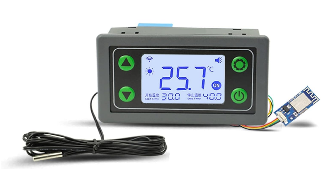
Figure 2: The thermostat highlighting its AC110-220V 30A power capability and remote WIFI control feature.
