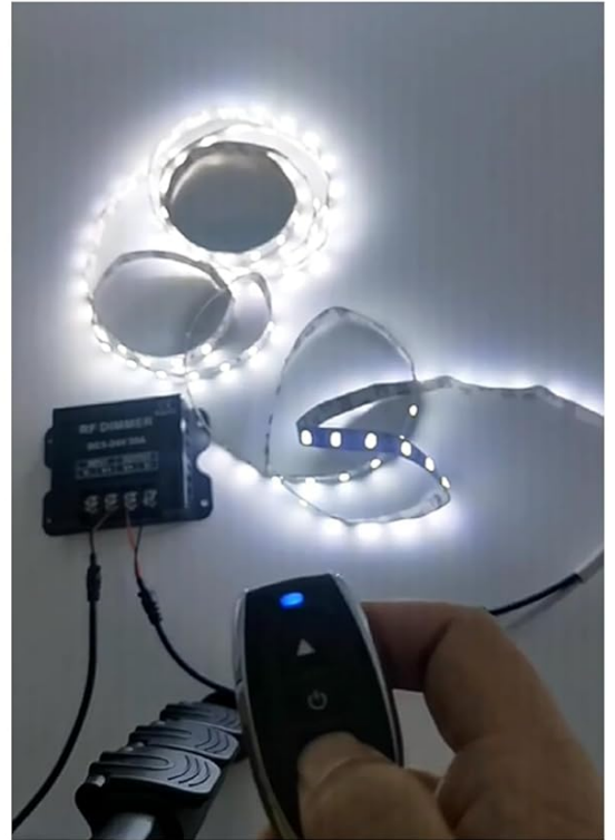
Figure 5.1: Illustration of the dimmer unit connected to an LED strip and power supply, demonstrating the wiring process.
