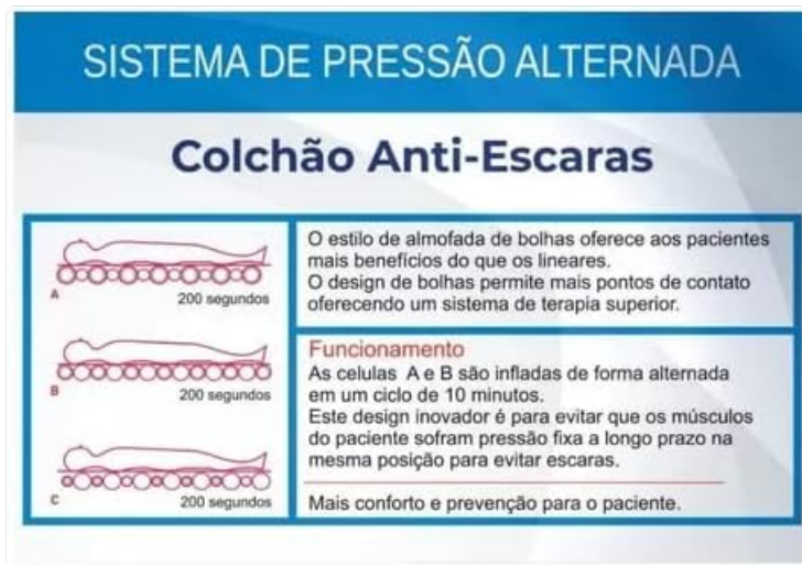
Image 3: Diagram showing the alternating inflation and deflation of air cells (A, B, C) over a 200-second cycle, demonstrating how the system prevents prolonged fixed pressure.
