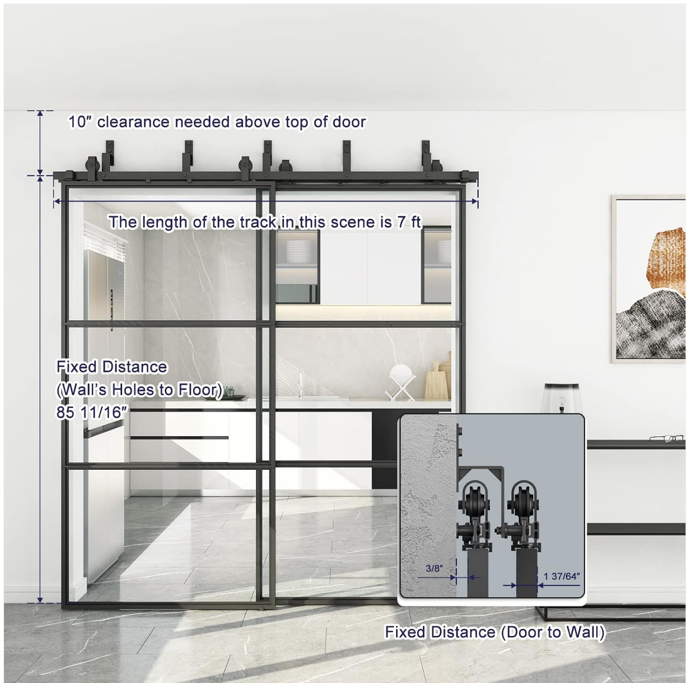
Image: A detailed diagram illustrating the necessary 10-inch clearance above the door, the 7-foot track length, and the fixed distances from the wall to the door and from the wall's mounting holes to the floor.
