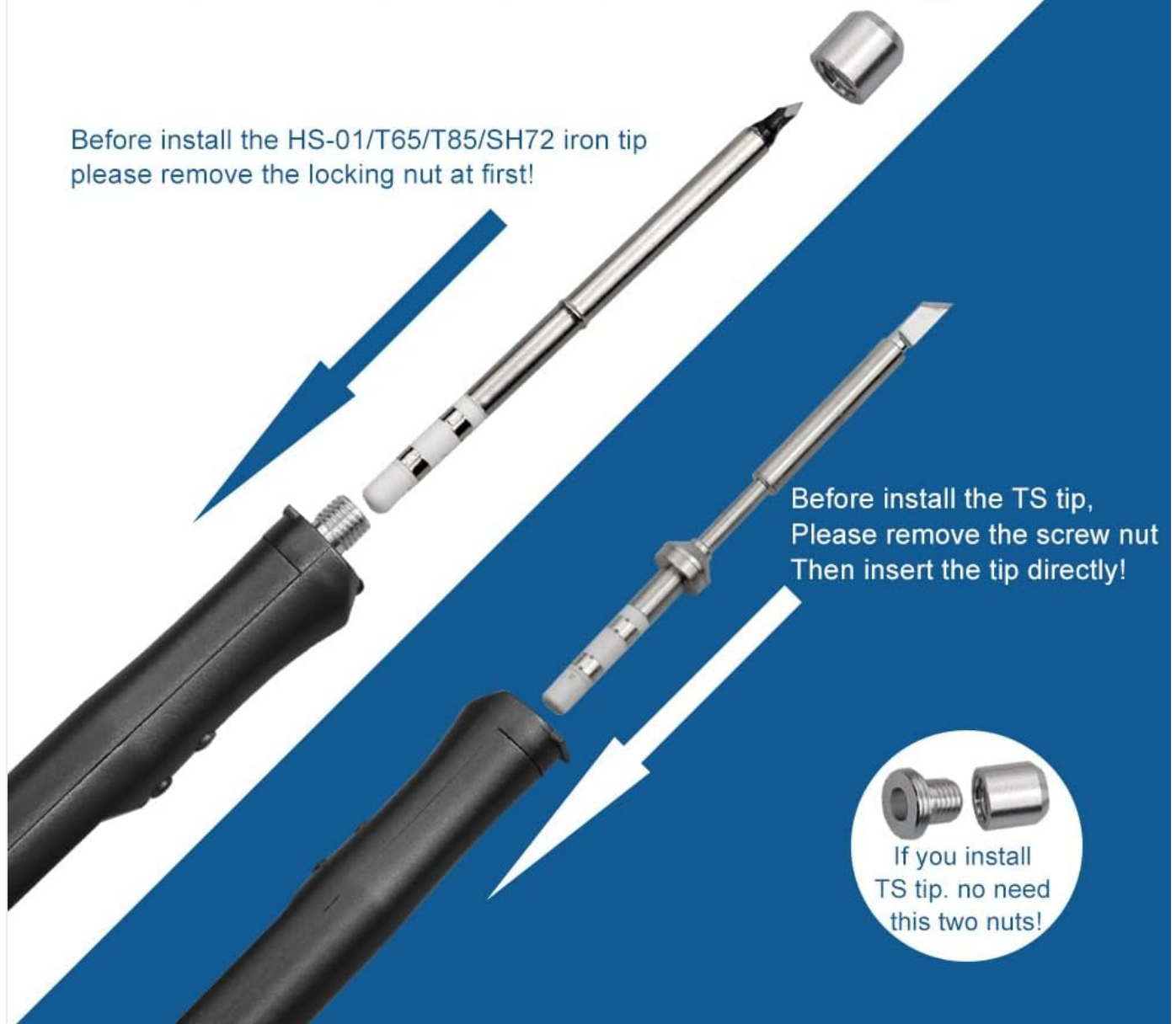
Image 5.1: Guide for installing different types of soldering tips. This image illustrates the two methods for tip installation: one with a locking nut for HS-01/T65/T85/SH72 tips and direct insertion for TS tips.
