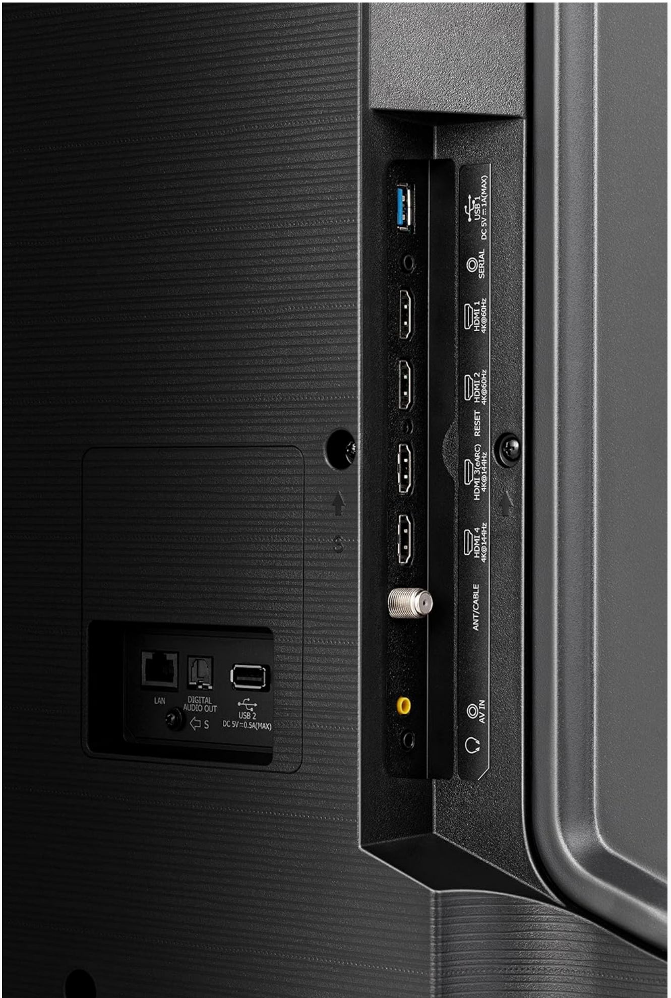
Figure 4: Side-facing connectivity ports on the 65U7K TV.
