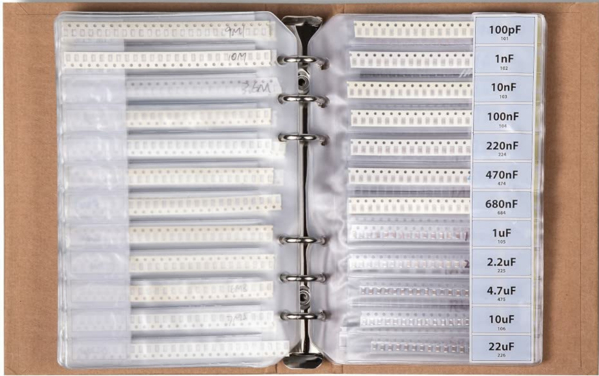
Figure 4: A section of the book dedicated to capacitors, showing different values.
