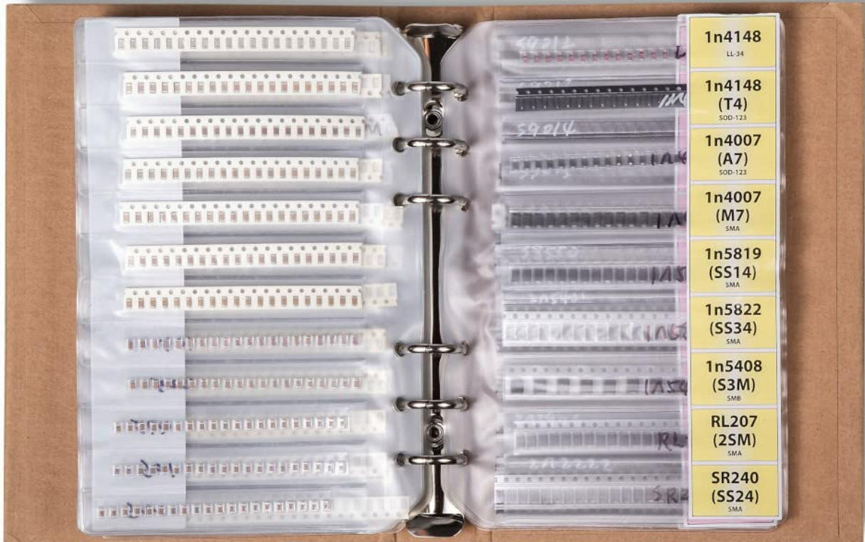
Figure 5: A section of the book dedicated to diodes, showing different types and values.
