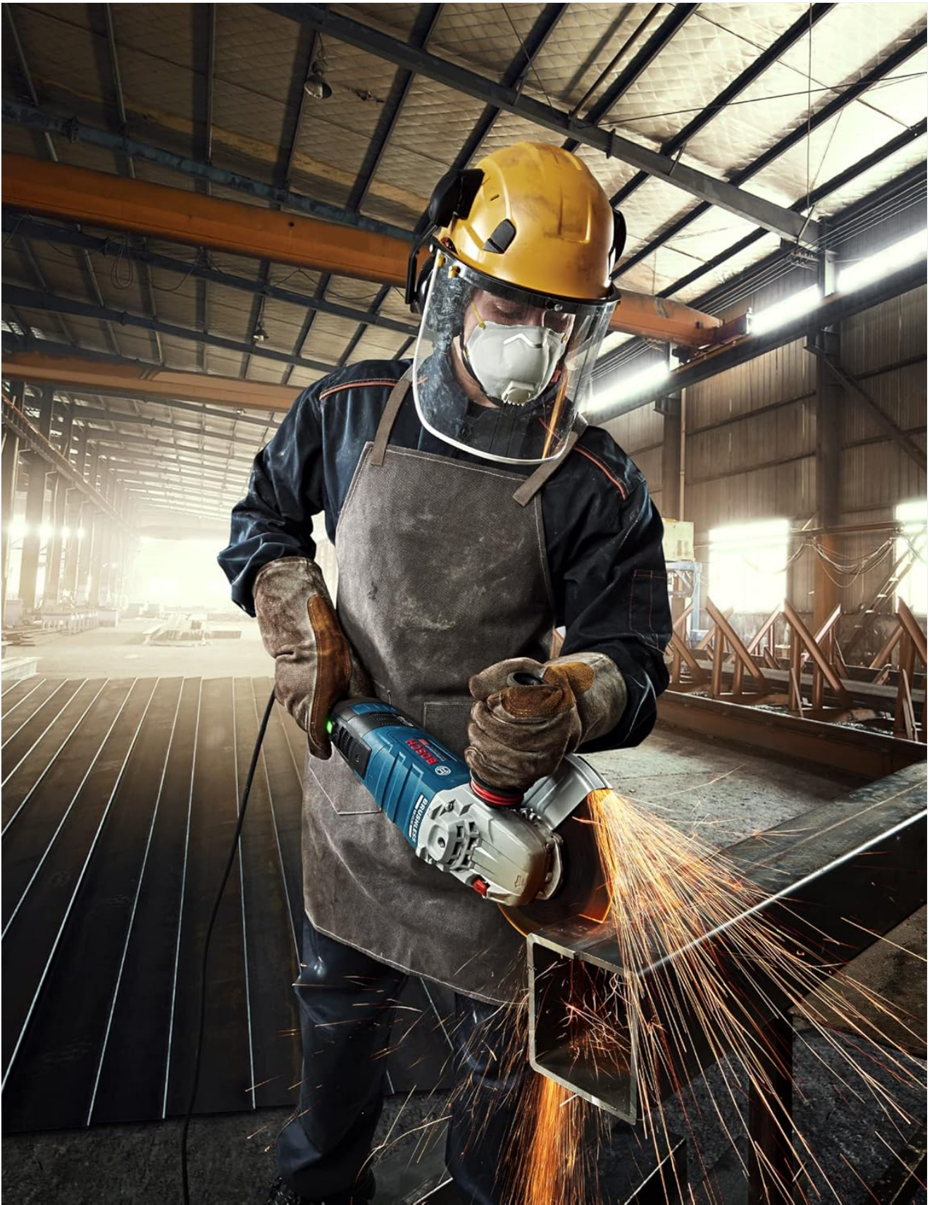
Image 3: A worker demonstrating safe operation of the Bosch Professional GWS 30-230 B Large Angle Grinder, wearing a hard hat, face shield, respirator, hearing protection, protective clothing, and gloves. Sparks are visible during the grinding process.
