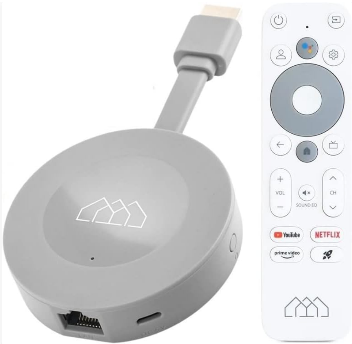
Image: A close-up view of the Homatics DONGLE G, highlighting its HDMI connector, USB-C port, and RJ45 port, alongside the voice remote control.
