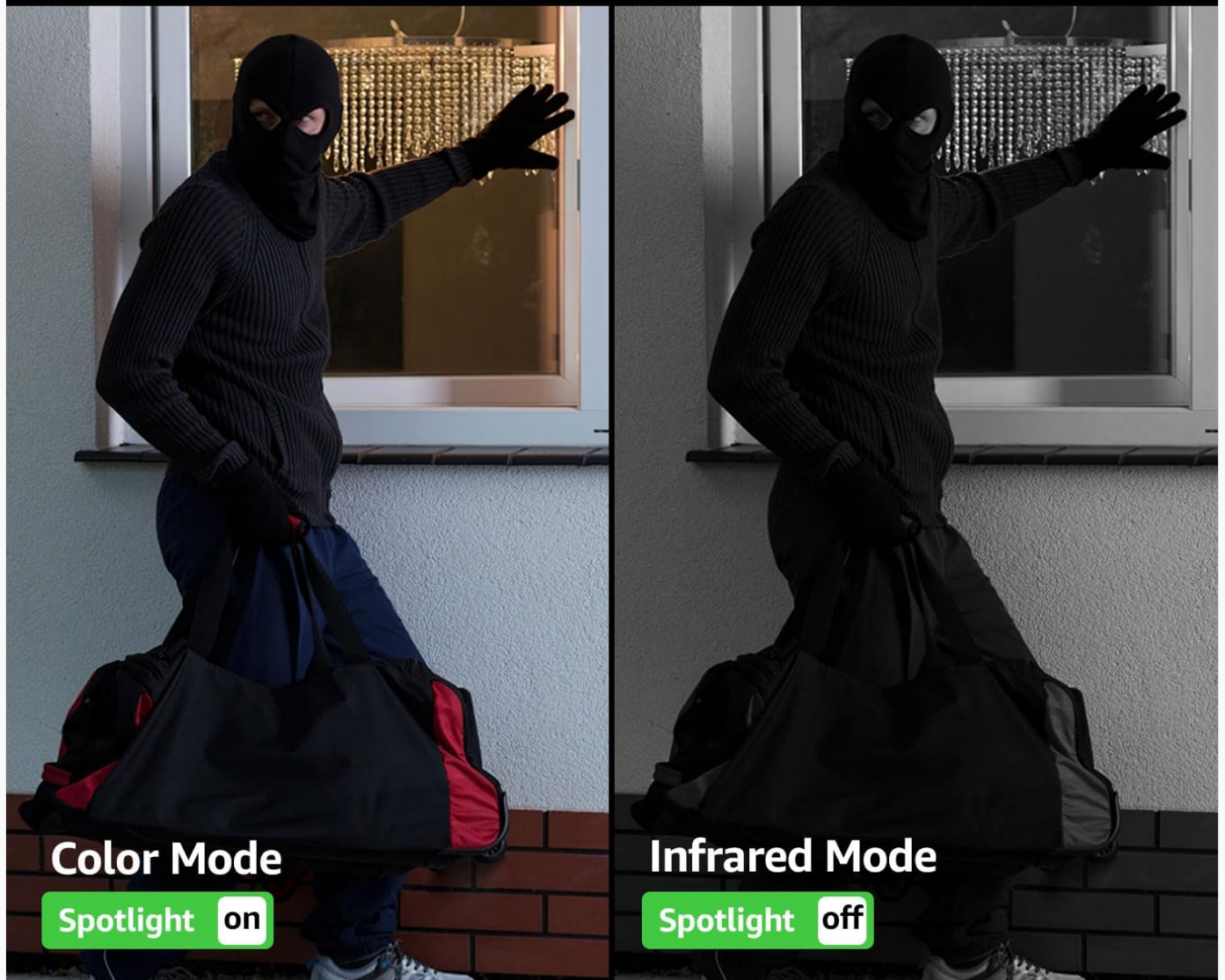
Image: A side-by-side comparison showing the difference between Color Mode (spotlight on) and Infrared Mode (spotlight off) at night, highlighting the camera's versatile night vision capabilities.
