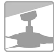
Sloped Ceiling \leq 20^\circ
