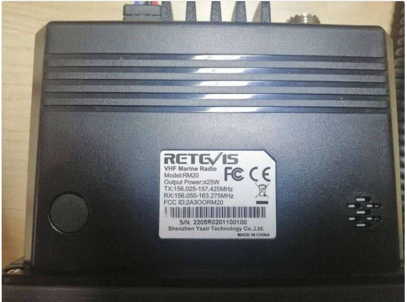
Image: The rear panel of the Retevis RM20 marine radio, displaying the product label with model number, output power, frequency range, and FCC ID.
