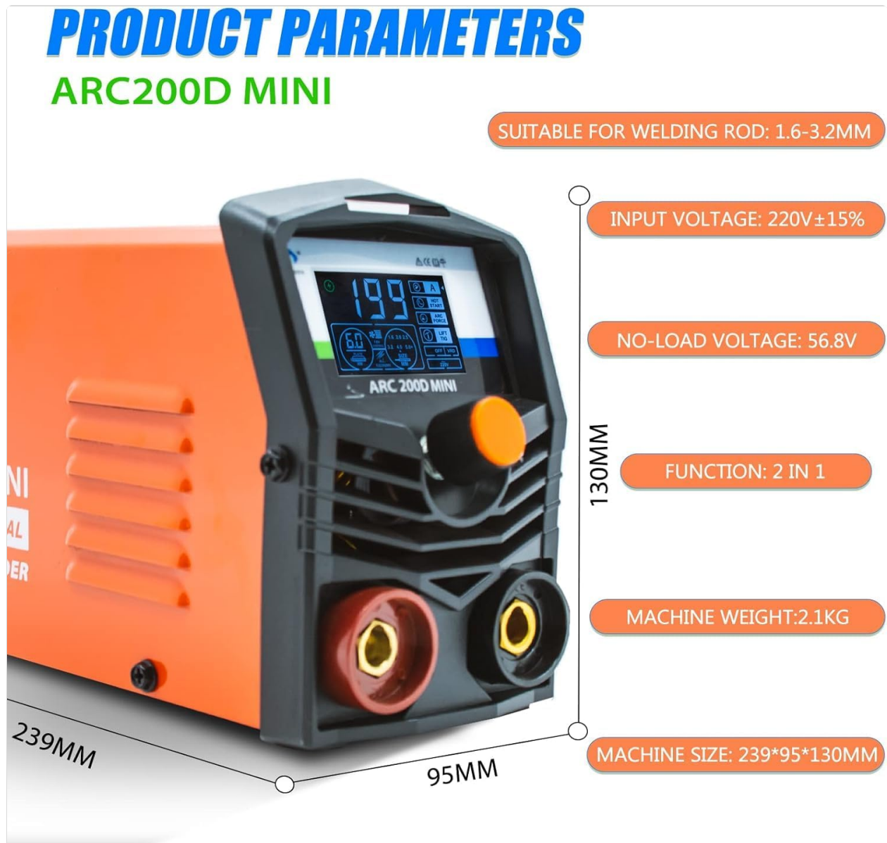
Figure 7.1: Product parameters and dimensions of the ARC200D Mini.
