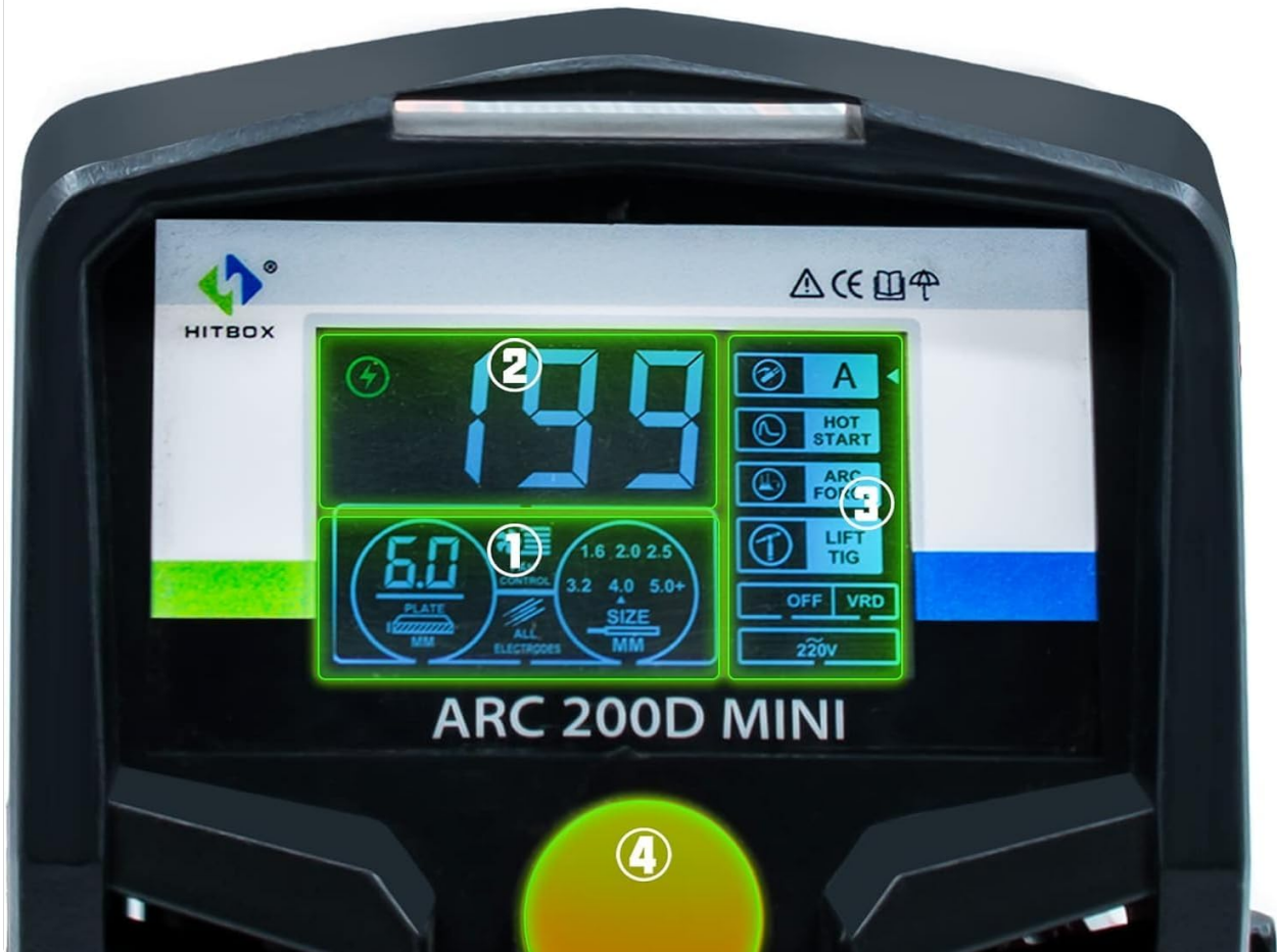
Figure 2.2: Front panel introduction of the ARC200D Mini, highlighting the digital display and control knob.
