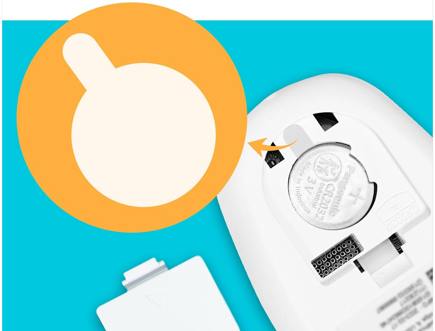
Image 3.1: A close-up view of the Easy@Home Blood Glucose Monitor, showing the battery compartment and the insulating tab being removed.
