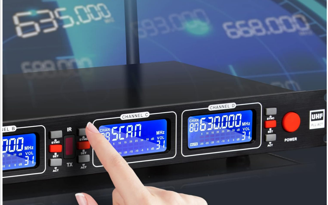
Image 3.2: Close-up of the receiver showing the 'SYNC' button and IR sensor for one-key pairing.
