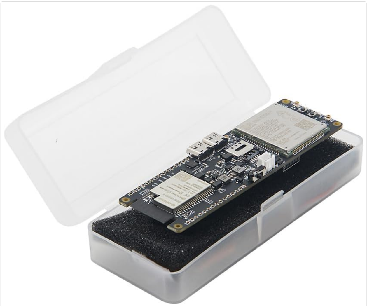
Figure 2: Top view of the LILYGO T-SIM7600G-H board, showing the ESP32 module, SIM7600G module, dual USB-C ports, and Nano SIM slot.
