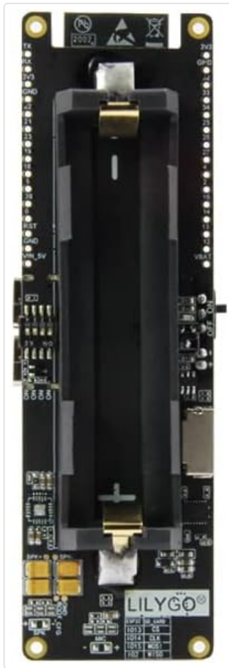
Figure 5: Top view of the LILYGO T-SIM7600G-H board, highlighting the 18650 battery holder. Ensure correct battery polarity during installation.
