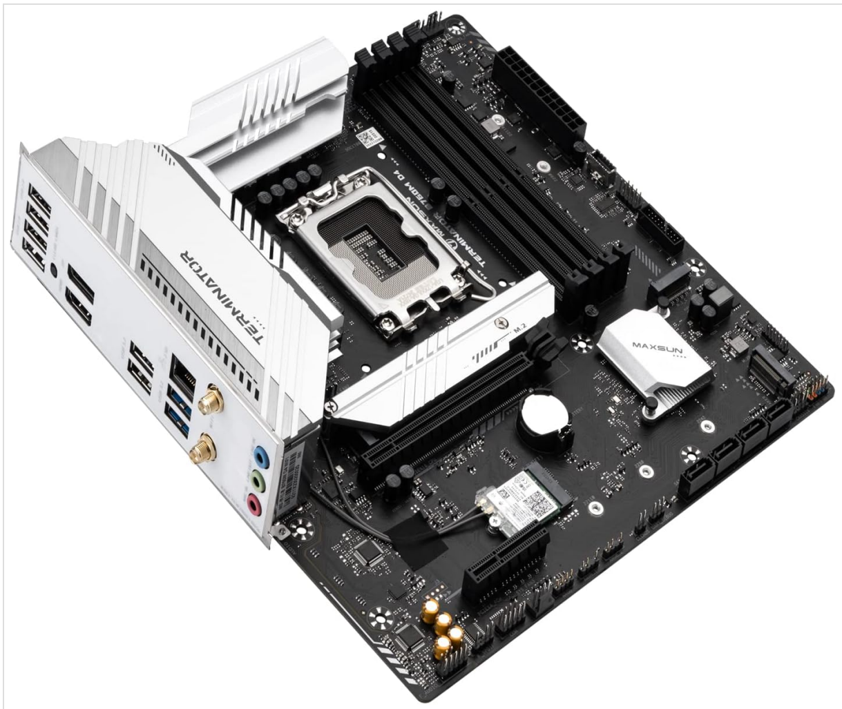
Figure 4.3: Angled view of the motherboard, illustrating the placement of the M.2 slots and the chipset heatsink.
