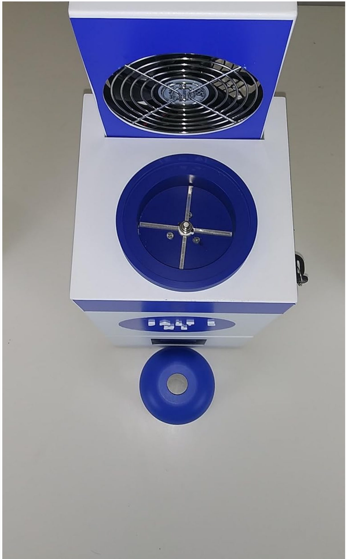
Figure 4.2: Top view of the halogenerator showing the salt chamber.
