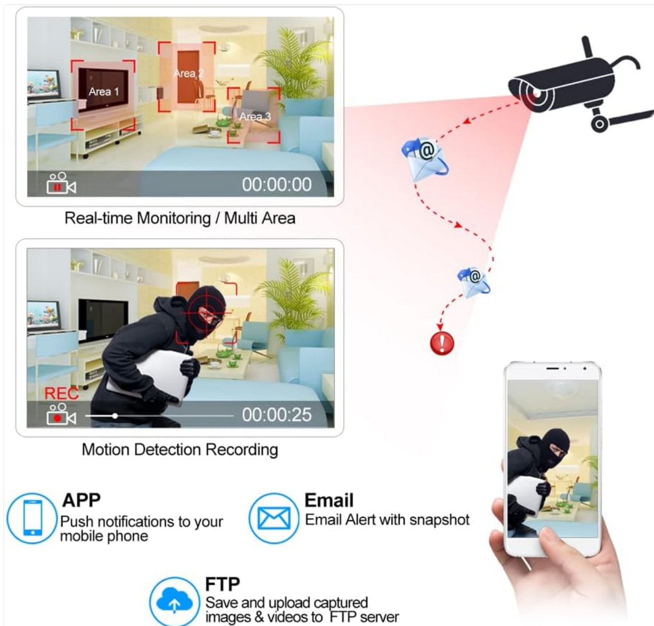
Figure 3.3: Motion Detection and Alert System. This diagram illustrates how the NVR detects motion within defined areas, triggers recording, and sends push notifications or email alerts to the user's mobile device.
