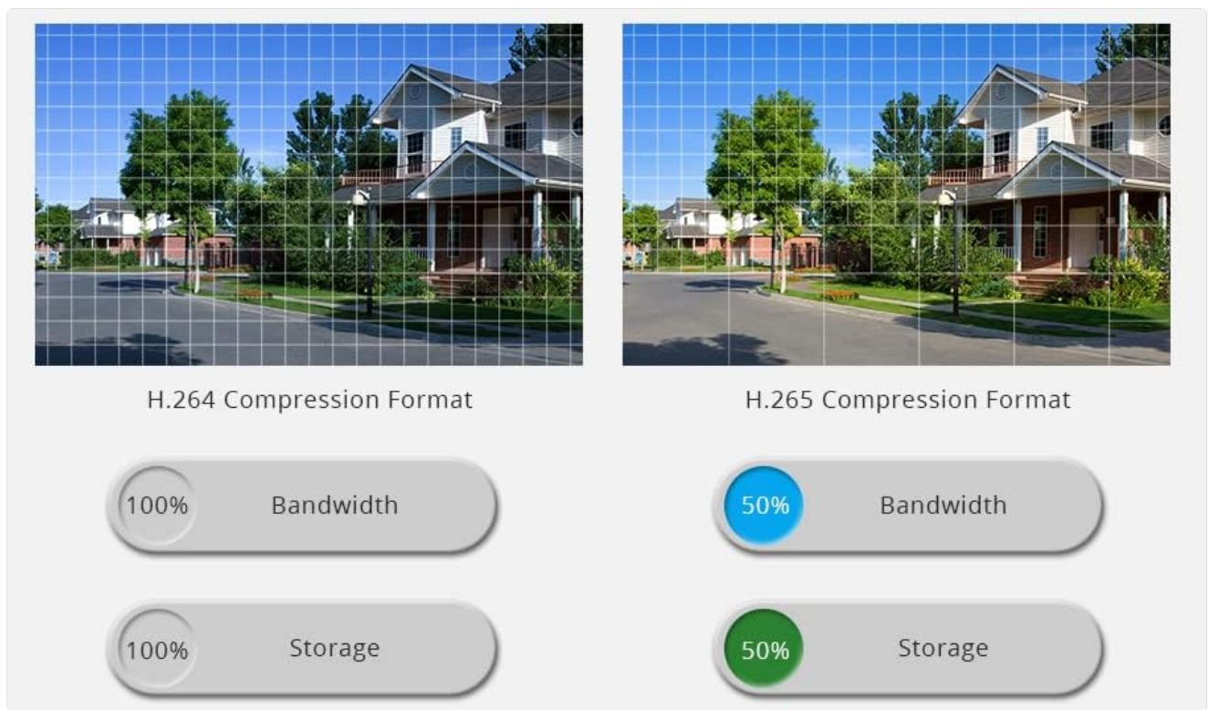
Figure 3.2: H.264 vs. H.265 Compression Efficiency. This visual comparison highlights how H.265 achieves similar video quality with significantly less bandwidth and storage requirements compared to H.264.
