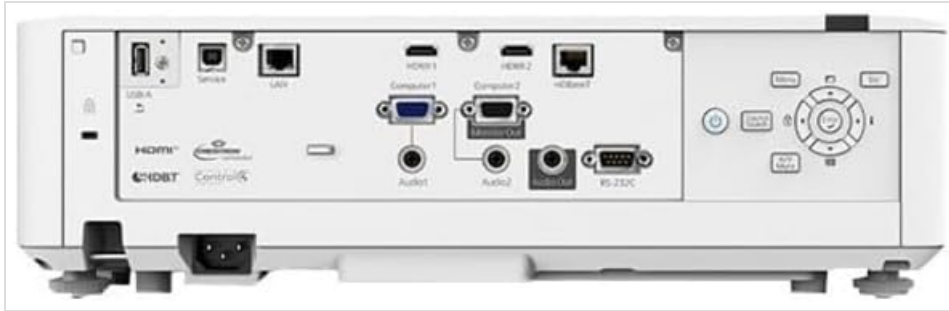
Image 2: Rear panel of the Epson PowerLite L520U projector, showing various input and output ports. These include HDMI, USB-A, USB-B (Service), LAN (RJ-45), Computer (VGA) inputs, Audio inputs/outputs, and RS-232C for control. The power inlet is also visible.
