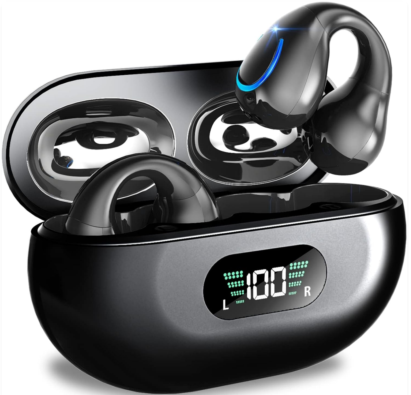
Figure 3.1: Kinganda Q71 Clip-On Open Ear Headphones and Charging Case. The earbuds are securely nestled in the charging case, which features a digital display indicating battery levels.
