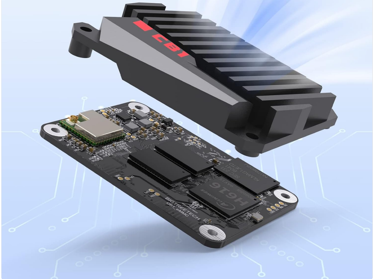
Figure 3.8: CB1 eMMC Heat Sink Compatibility.
