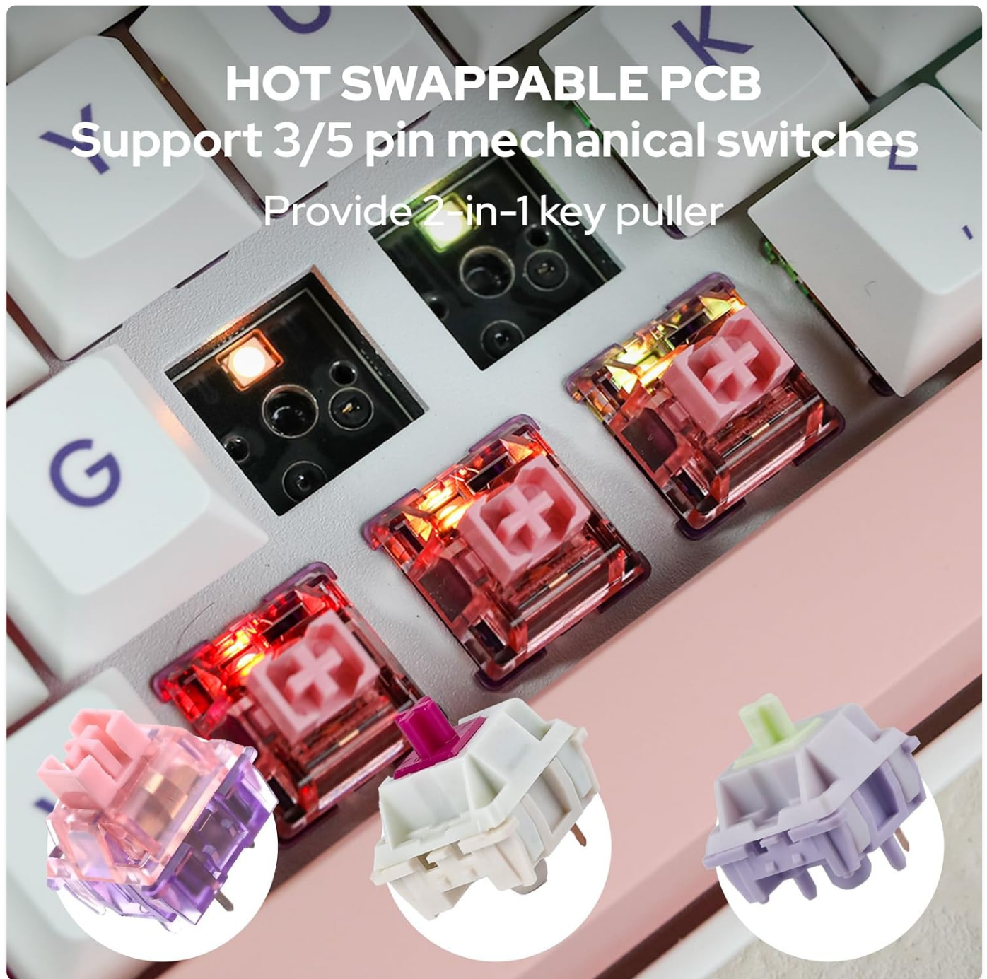
Figure 7: Hot-swappable switch sockets on the PCB.
