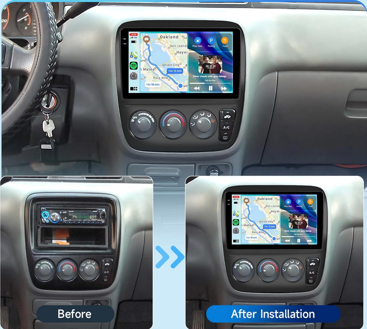
Image: Visual comparison of the dashboard before and after the car stereo installation.
