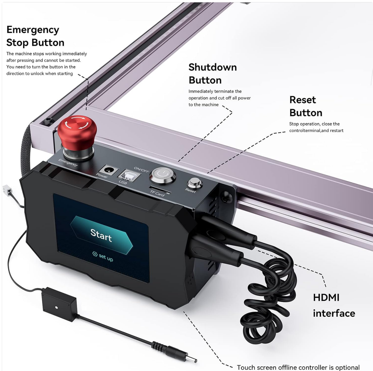
Image: The AIC1 control box featuring an optional touchscreen controller connected via HDMI, illustrating the offline control capabilities and the emergency stop and reset buttons.
