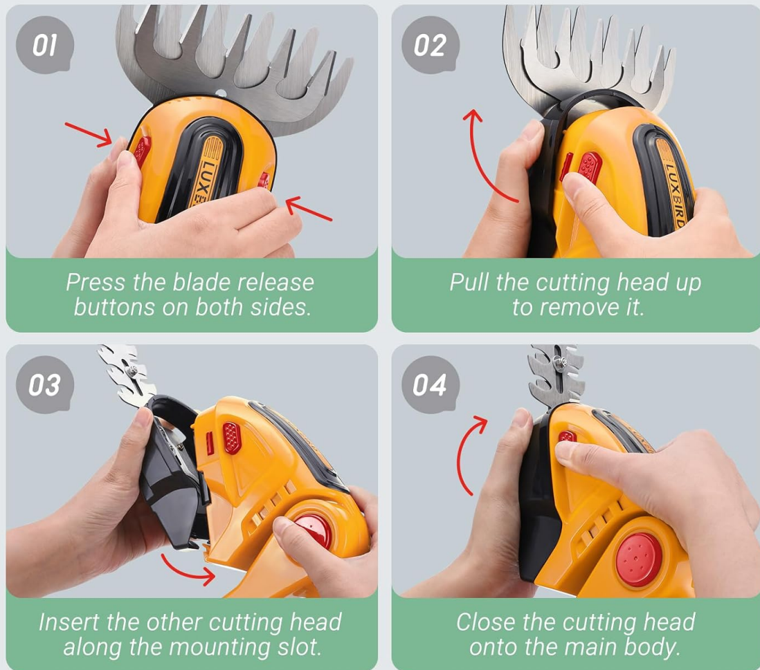
Figure 5: Step-by-step guide for replacing the cutting head.
