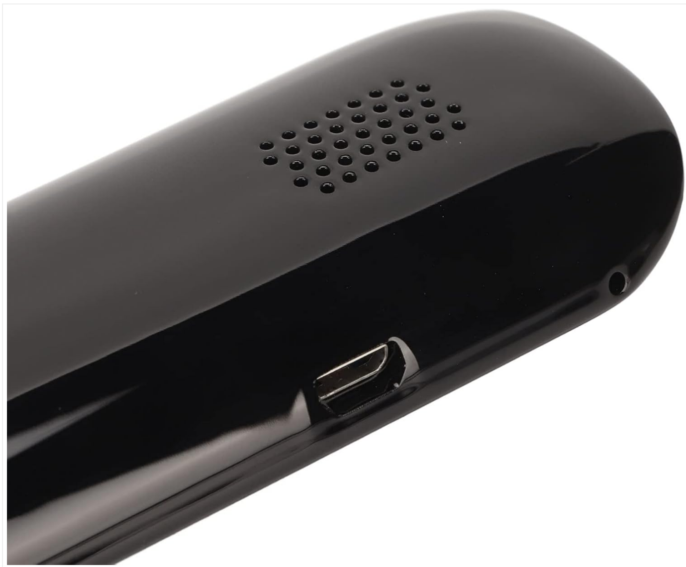
Image: Bottom view of the G5 PRO translator, showing the micro USB charging port and speaker grille.
