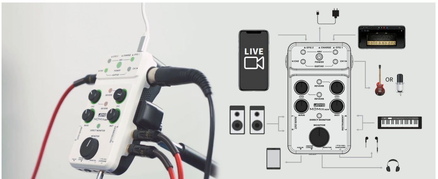
Figure 7: Connection diagram for the MOMIX PRO, illustrating various input and output possibilities.
