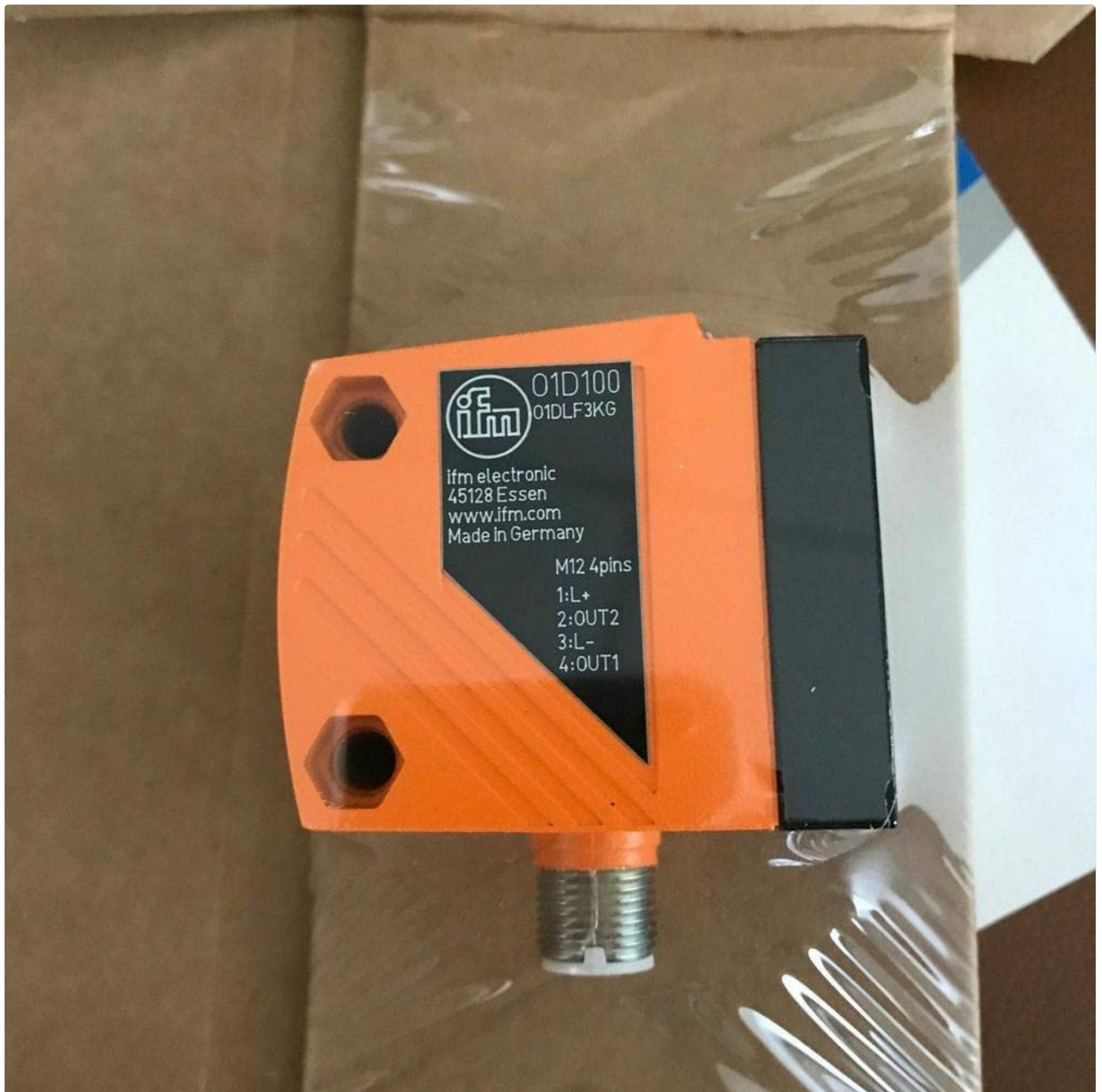
Figure 1: Front view of the O1D100 sensor, highlighting the M12 connector and pinout details. This image shows the sensor's main body, the label with model information and electrical connections, and the threaded M12 connector at the bottom.
