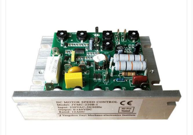
**Figure 3.1:** Generic JYMC-220B-I Lathe DC Brushed Motor Speed Control Board. This image displays the top view of the control board, highlighting its electronic components, heatsink, and the label indicating model number, input/output specifications, and CE certification.
