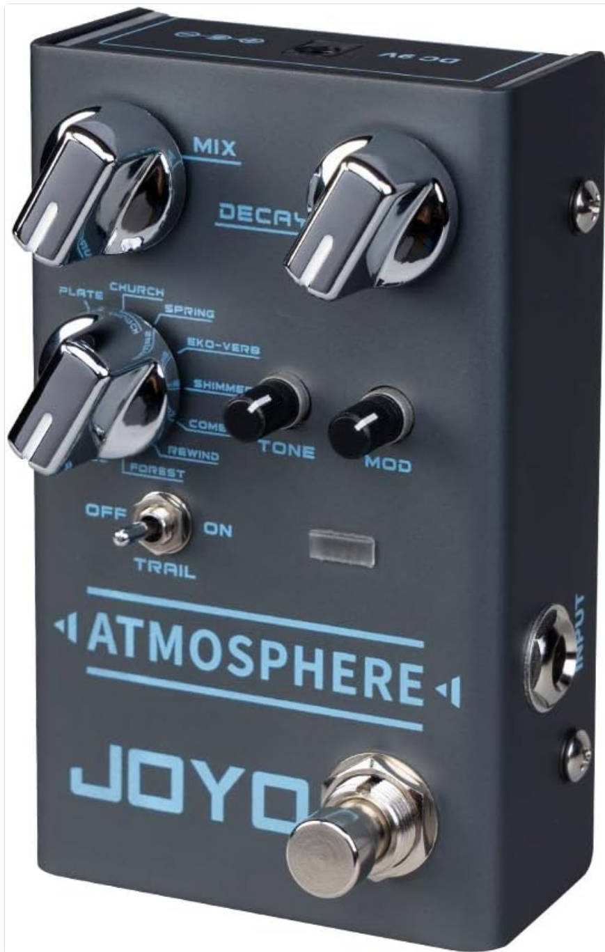
Image: Top view of the JOYO Atmosphere R-14 pedal, showing the MIX, DECAY, TONE, MOD knobs, the 9-position reverb type selector, the TRAIL switch, and the footswitch.
