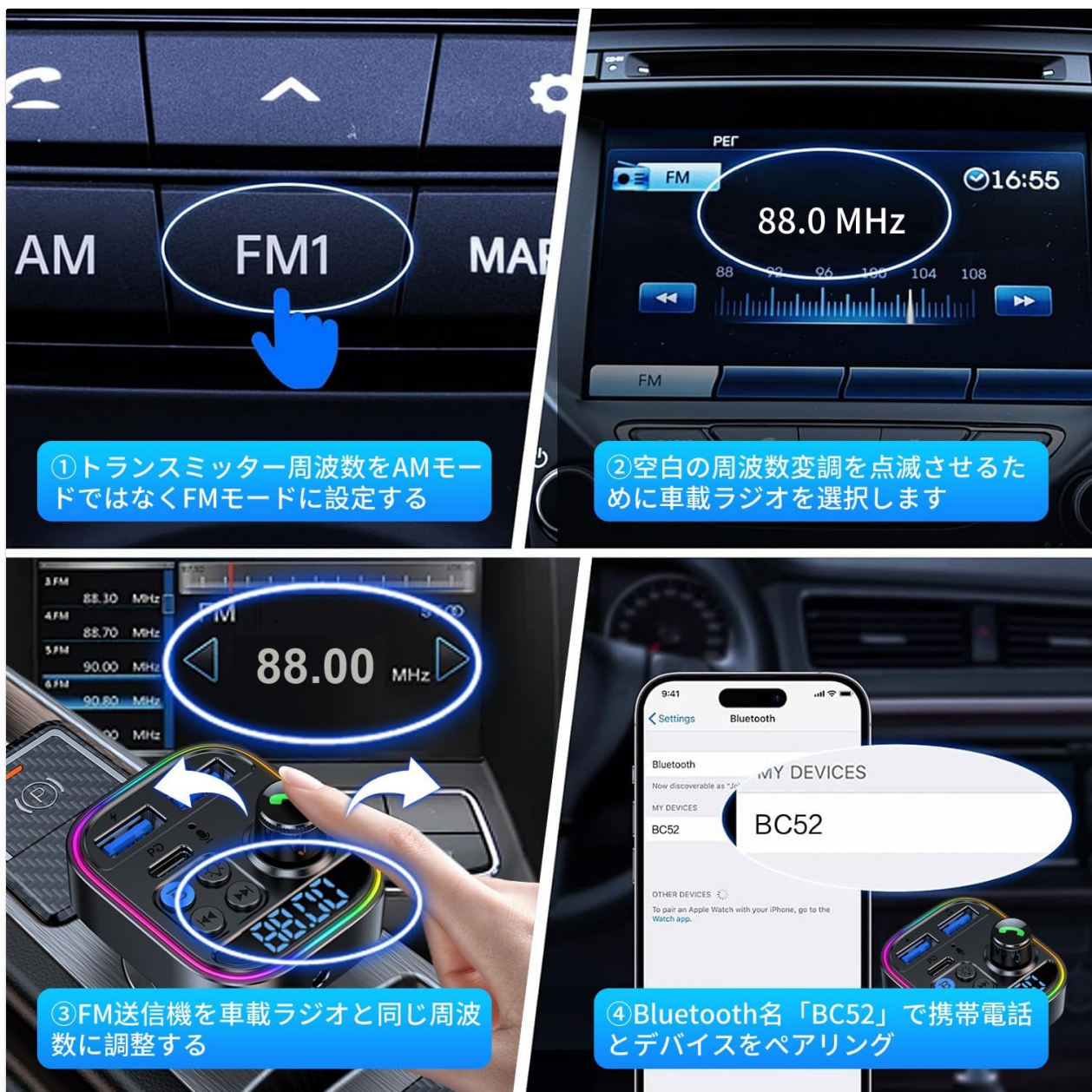
Image 3.1: Visual guide for setting up the FM transmitter, including tuning the car radio and pairing via Bluetooth.
