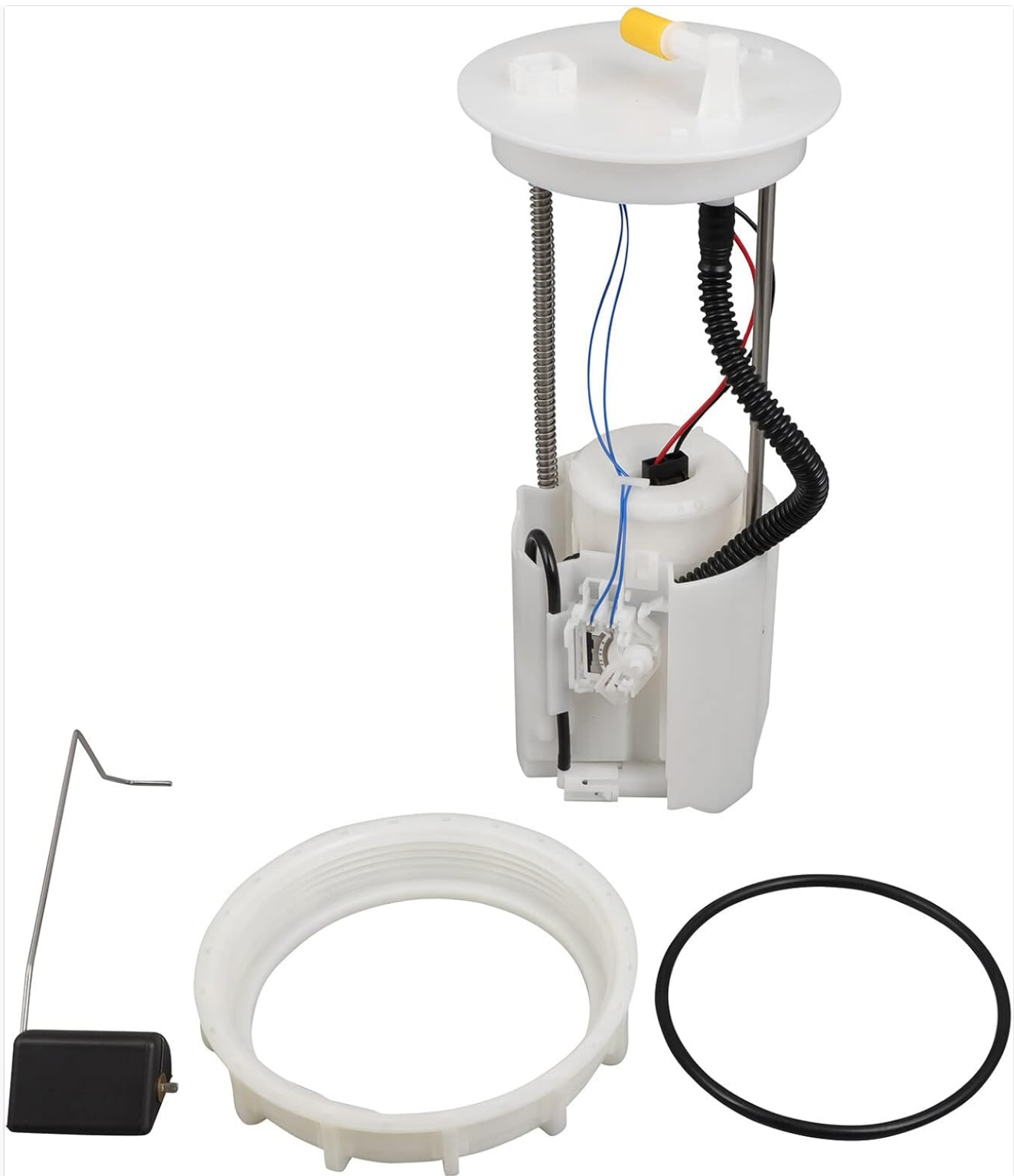
Image 1.1: ECCPP Electric Fuel Pump Module Assembly. This image displays the complete fuel pump module, including the pump, fuel level sender, and associated wiring and hoses.
