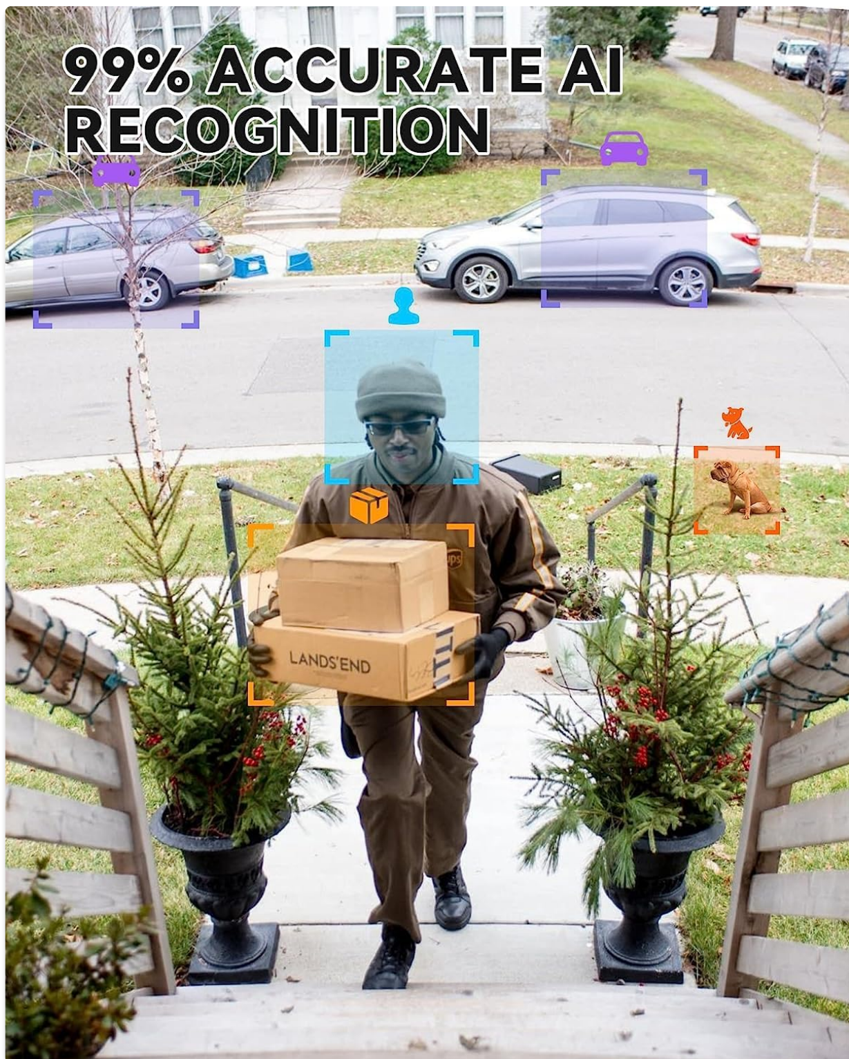
Image: The doorbell camera's AI recognition feature identifying and outlining a delivery person, a car, and a dog in its field of view.
