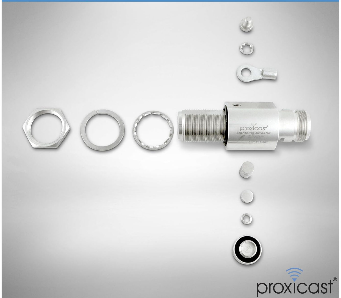
Figure 3.3: Individual components of the lightning arrester, including the main body, replaceable gas discharge tube, O-ring, lock washers, and ground wire terminal lug.
