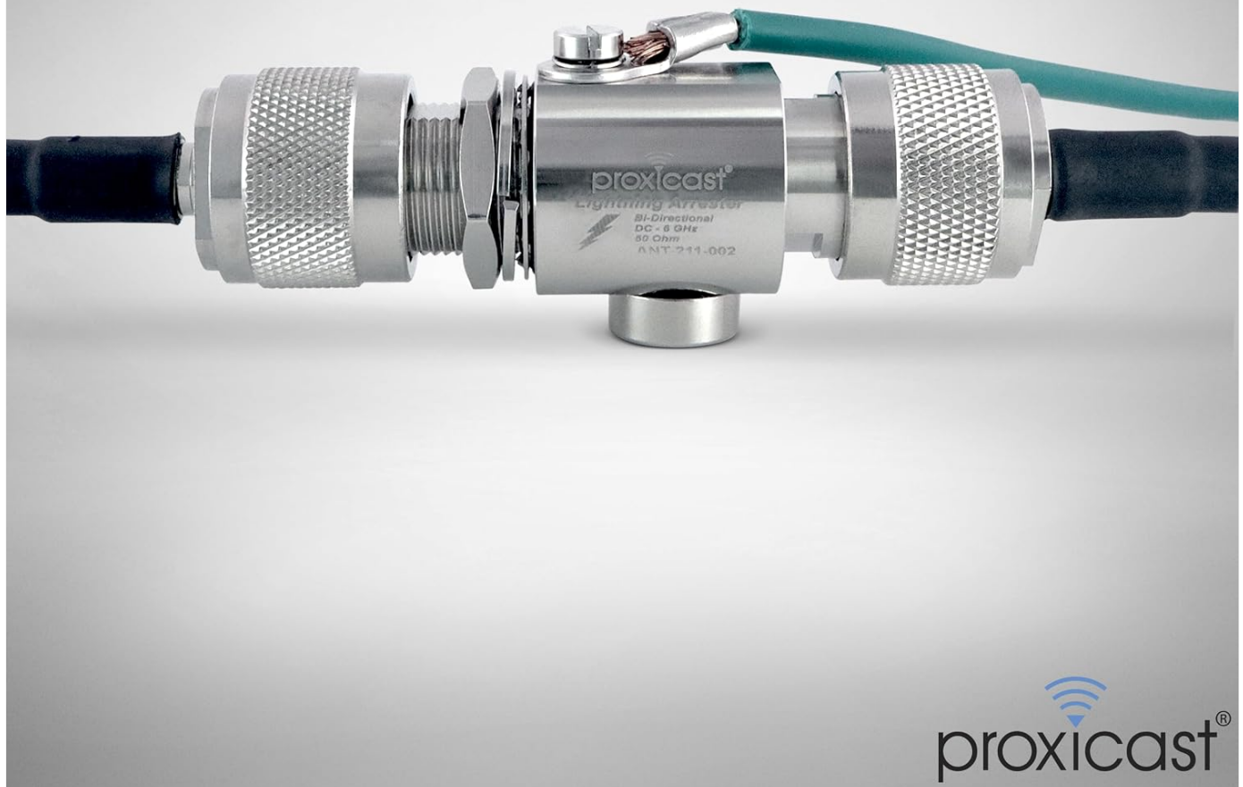
Figure 3.2: The lightning arrester connected in-line with two coaxial cables. Ensure all connections are secure and the ground wire is properly attached to the terminal lug.
