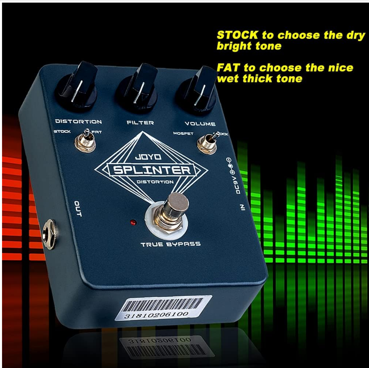
Image 2.2.2: JOYO Splinter Distortion with STOCK/FAT switch explanation.
