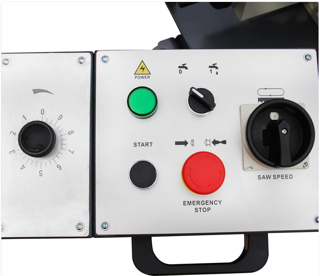
Figure 3.1: Close-up of the control panel. This image shows the various buttons and dials for operating the band saw, including power, start, emergency stop, and saw speed selection.
