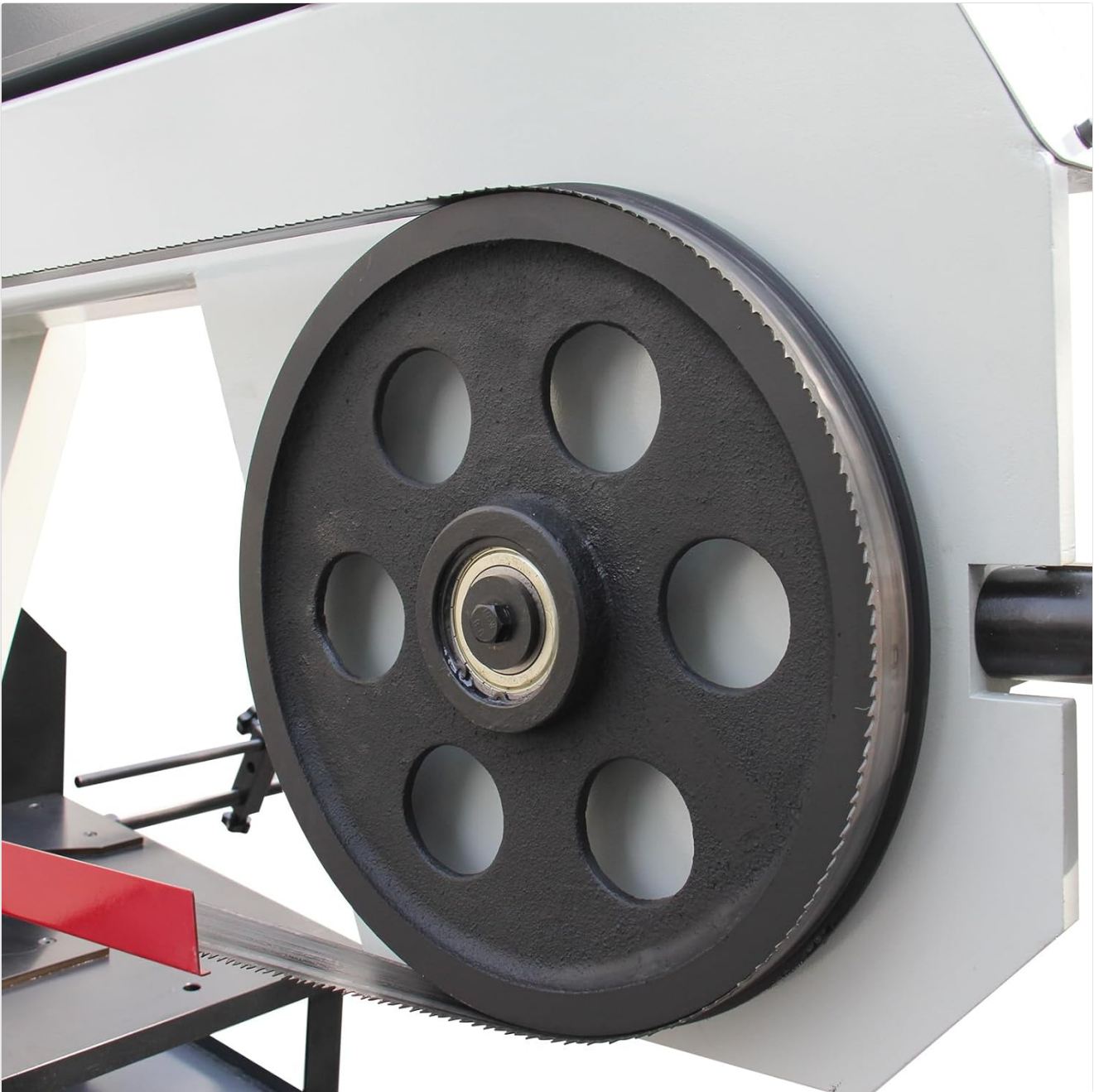
Figure 4.1: Detail of the blade wheel and blade path. This image shows the mechanism that drives the band saw blade, emphasizing the importance of proper blade alignment and tension.
