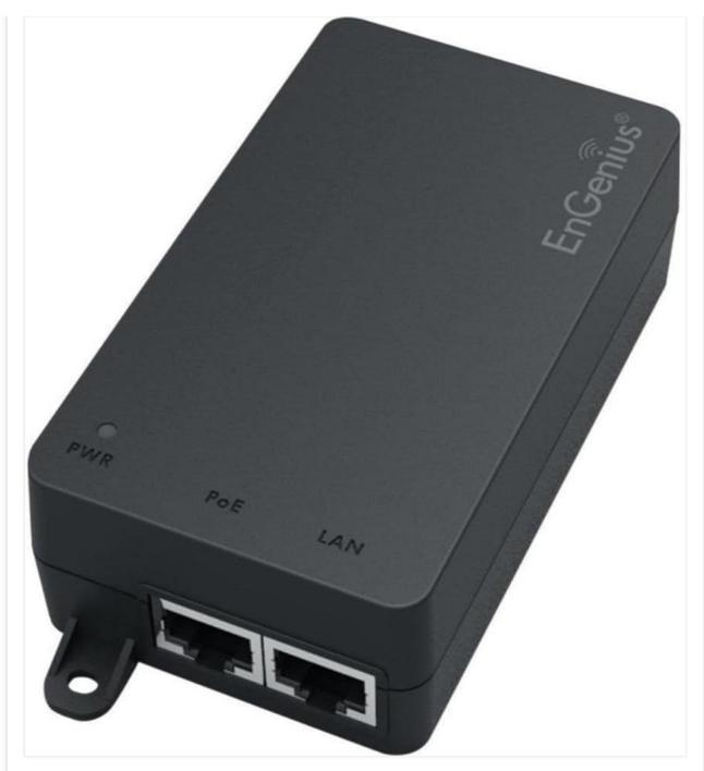
This image displays the EnGenius Gigabit Proprietary PoE Adapter, highlighting its compact black casing and the labeled PWR (Power), PoE (Power over Ethernet), and LAN (Local Area Network) ports. The EnGenius logo is visible on the top surface.
