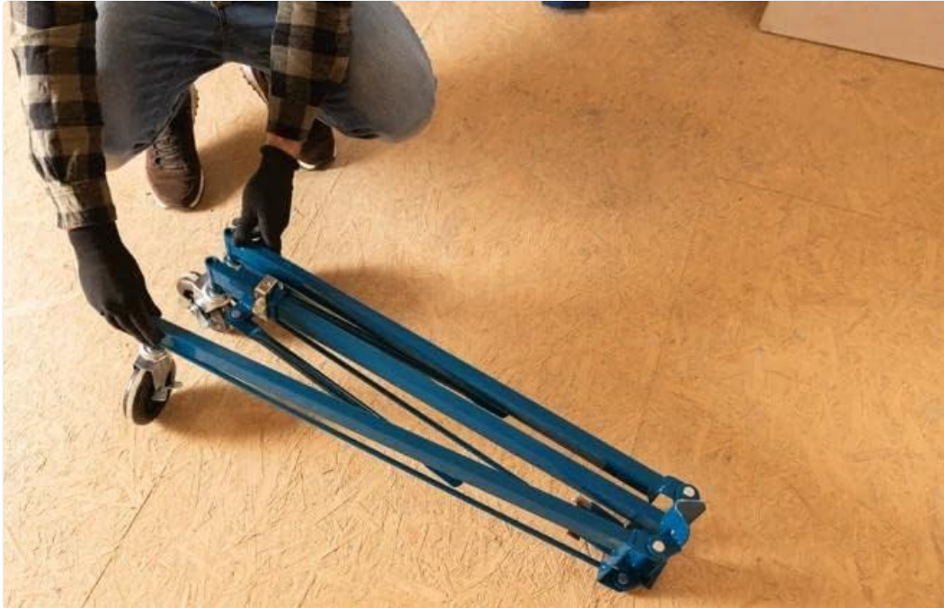
Figure 2: The panel lift disassembled into its main components for compact storage and transport.
