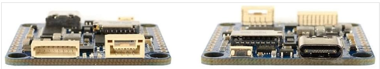
Figure 4.4: Side views of the MATEKSYS H743-SLIM V3 Flight Controller, illustrating the various connectors such as the USB Type-C port, JST-SH1.0_8pin, and JST-GH1.25_4pin connectors.
