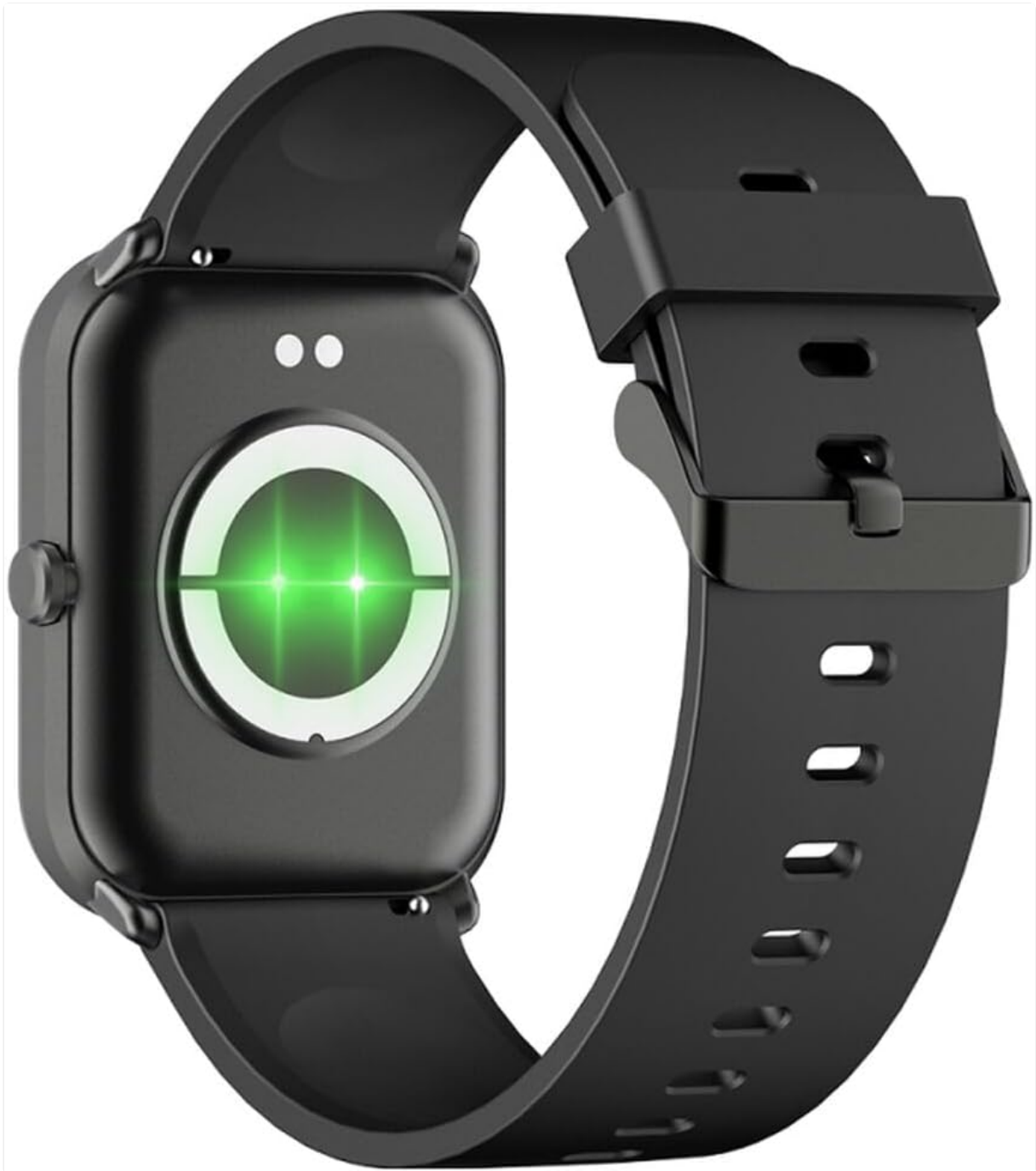
Figure 2: Rear view of the smartwatch, highlighting the charging contacts and health sensors.
