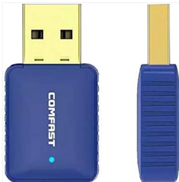
Figure 3: Front and side view of the COMFAST CF-726B adapter. This perspective shows the overall dimensions and the blue LED indicator light.
