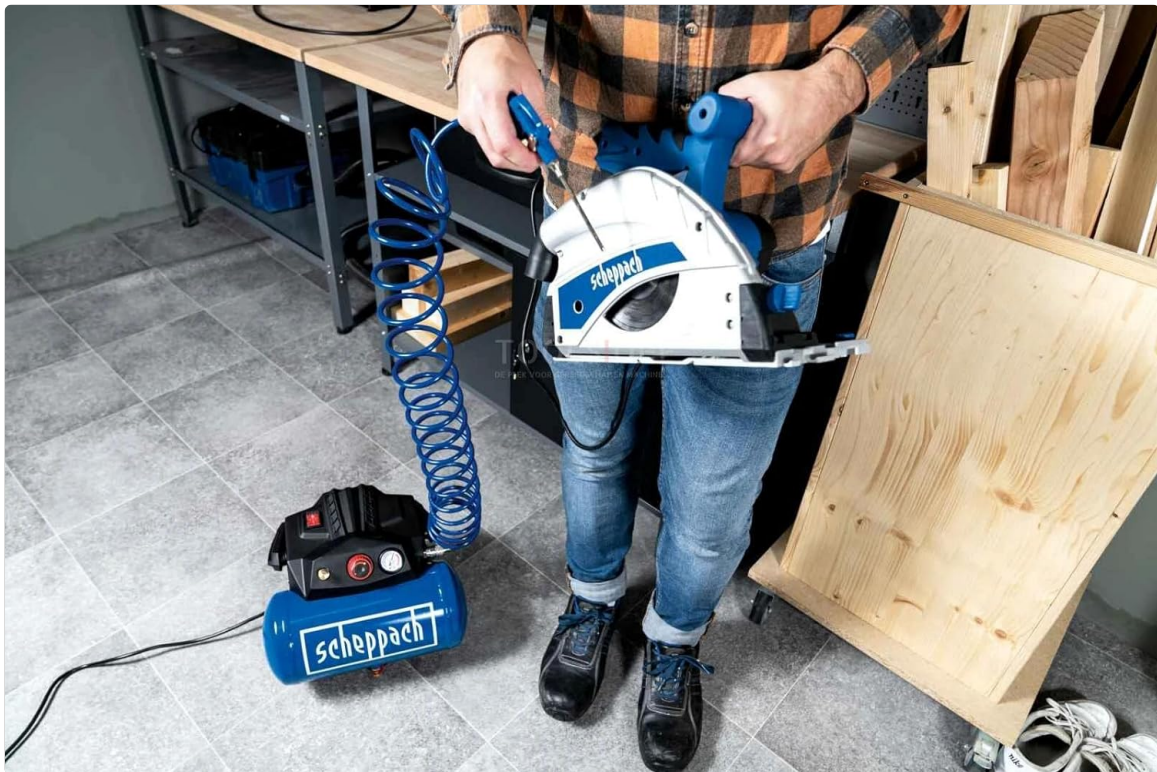
Figure 5: The HC06 can power various pneumatic tools, such as this circular saw.
