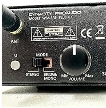
Image: A close-up view of the Receiver's mode switch (Stereo, Bridge, Mono) and the volume control knob.
