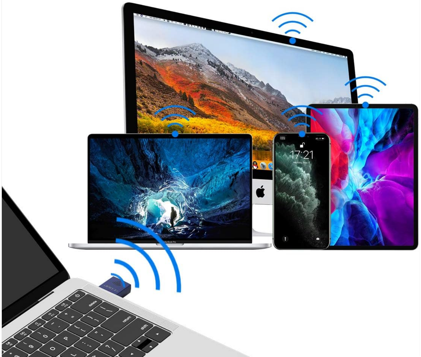
Image 3.2: Illustration of the Soft-AP mode, demonstrating how the USB WiFi adapter enables a computer to share its internet connection with other devices like laptops, tablets, and smartphones.
